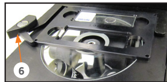
Mechanical stage with vessel holder secured by stage clip 6
