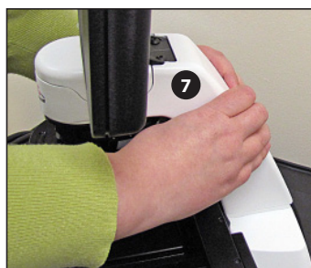
Grasp under support arm ❼ with both hands to lift EVOS
