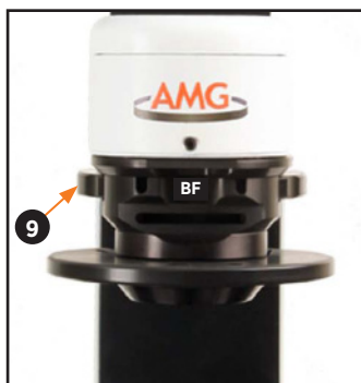
Phase turret ⑨ (side and front views) in BF position
