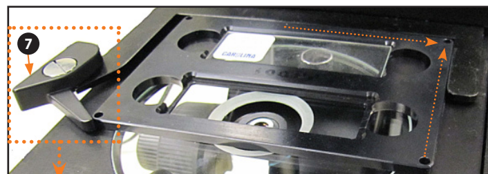
Vessel holder secured by stage clip ⑦
